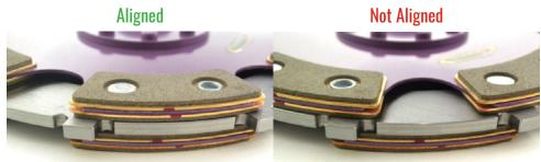
8. Mount the main pressure plate casting into the adapter ring with the fulcrum facing up. At this point use the alignment tool to align the friction discs to the pilot bearing.
