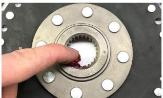
6. Locate the "Transmission Side" marking on the friction discs.
