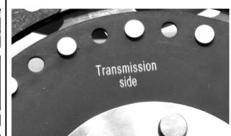
7. Install the bottom disc on the flywheel with the "transmission side" facing away from the flywheel followed by an intermediate plate. Install the top friction disc the same way. Ensure that all parts are clean and that the orientation is correct. Double check that the discs are in the correct orientation by ensuring that there is a small amount of clearance between the hubs (0.5mm/0.020" or more).
