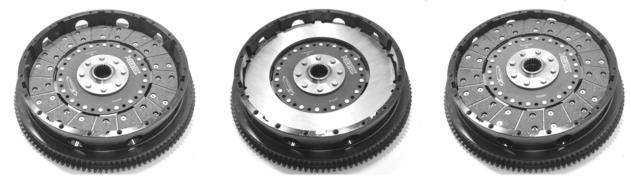
When ceramic button friction discs are used, ACS recommends aligning the buttons of the top disc with the bottom, however it is not critical.
