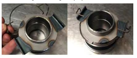
7) Connect the clutch fork to the release bearing carrier by tilting the fork under the clip so the clip sits in the grooves of the fork.
