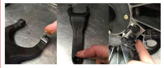
6) Install the release bearing clip onto the release bearing carrier. This clip only fits in one direction with the small tab on the bearing carrier holding the clip in place.
