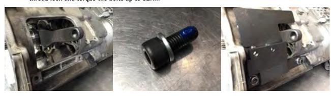
10) Use M8X1.25X20 bolts with spring washers to mount the slave cylinder in place on the adapter plate. Then install the new braided clutch line to the slave
