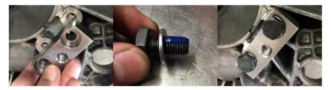
4) Use the new pivot ball supplied and install it onto the pivot ball bracket using thread lock. Torque it up to 70Nm.
