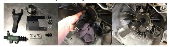
3) Use the pivot ball bracket and fix it to the transmission using the M10X1.25X20 bolts supplied along with the spring washers and thread lock. Ensure that the bracket is mounted in the correct orientation with the small chamfered edge facing upward. Torque the bolts up to 50Nm.
