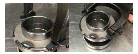
8) Lubricate the nosecone on the transmission and slide the release bearing and fork into place. Clip the clutch fork onto the pivot ball with a firm push.
