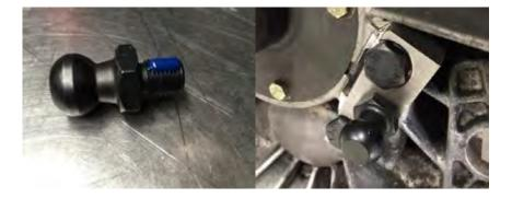
5) Using high temperature bearing grease, lubricate all the points of contact on the fork. This includes where it contacts the bearing carrier, push rod and pivot ball.
